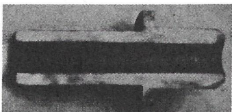
Cut-away view of a knurled valve guide (© Petersen Publishing Co.)
