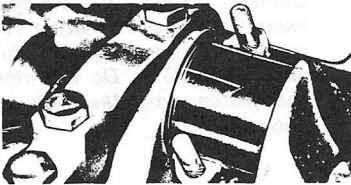
Plastigage installed on connecting rod bearing journal (© Chevrolet Div. G.M. Corp.)
